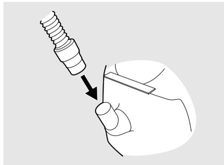
**2** Connect the other end of the patient tube to the mask and the ventilation valve, if applicable.
